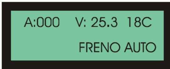
If the wind is very strong, the wind turbine may not stop completely, although the energy generated is diverted to the brake resistors.
