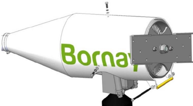
Next, the clamp bolt must be tightened at the back part of the nacelle.
