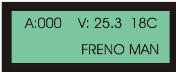
When the manual braking switch is activated, this is indicated on the screen at the end of the second line and the brake indication LED is also illuminated.
