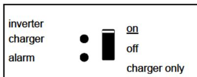
The AC input voltage is switched through and the charger is switched off. The battery charger can not reach battery end voltage (bulk protection mode).
