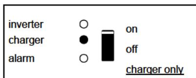
The AC input voltage is switched through and the charger operates in bulk or absorption mode.
