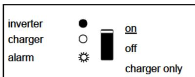
The inverter is switched on and supplies power to the load.
