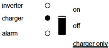
The AC input voltage is switched through and the charger operates in bulk or absorption mode.
