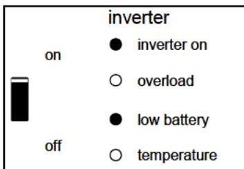
The inverter has switched off due to low battery voltage.
