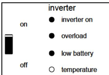
The inverter switched off due to excess ripple voltage on the battery terminals.
