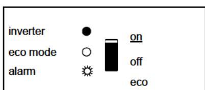
The inverter is switched on and supplies power to the load.
