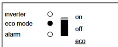
The inverter is switched on "eco mode" and supplies power to the load.
