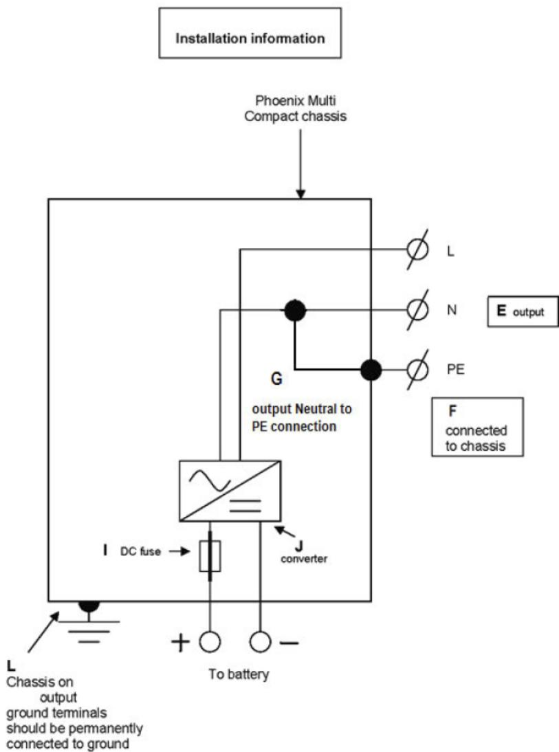
This ground wire "G" connects the output neutral to ground. It must be cut/removed if a floating output is required
