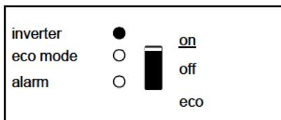
The inverter is switched on and supplies power to the load. Battery operation.
