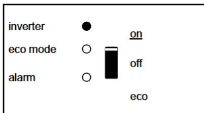
The inverter is switched on and supplies power to the load. Battery operation.
