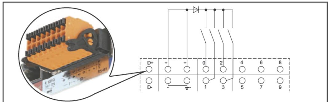
**Power supplied by an external power supply:**
