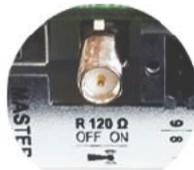
**IMPORTANT!** On an RS485 bus, the terminating resistor on the first and last devices must be active. For a detailed description, see the installation instructions.
