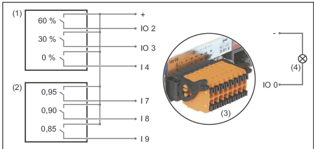
The ripple control signal receiver and the Fronius system monitoring connector are connected to one another by means of a four-pin cable in accordance with the connection diagram.
