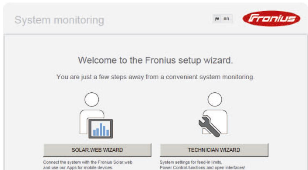
If you run the technician wizard, always remember to make a note of the assigned service password. This service password is necessary for making settings in the "System overview" and "EVU Editor" [UC Editor] menus as well as for advanced battery settings. If the technician wizard is not run, no specifications regarding power reduction are set and hybrid mode is not possible (charging and discharging of the Fronius Solar Battery).
