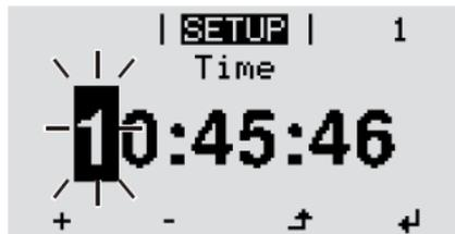
The current time appears. (HH:MM:SS, 24-hour clock), the "tens" digit for the hour will flash.
