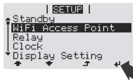
The inverter establishes the WLAN access point. The WLAN access point remains open for 1 hour.
